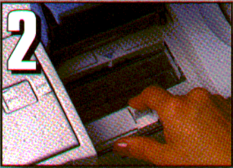
2 The Stampcreator PRO™ will instantly transfer the image you have prepared on your computer screen onto a transparent film, which will be loaded automatically from the magazine tray inside. 600 dpi thermal transfer printing will reproduce every detail from your graphics. Open the window and you will see the film (positive master) for your stamp positioned above the Xenon Flash Assembly.
